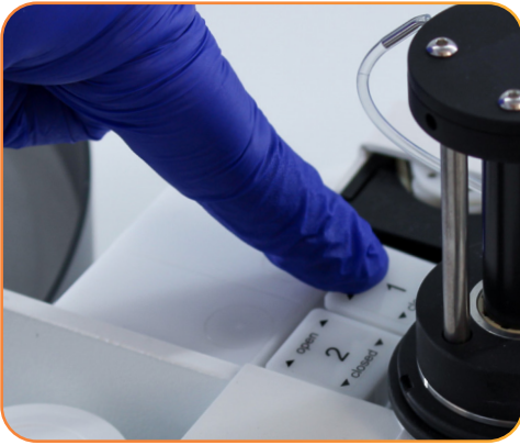
Figure 16 - Closing the sensor holder
