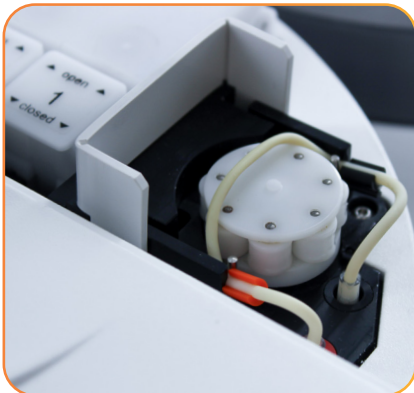
Figure 38 - Pump tube removed
