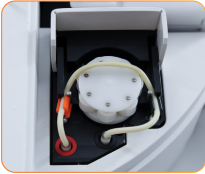
Figure 31 - push tube into the constriction
