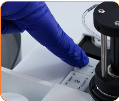
Figure 11 - Opening the sensor latch
