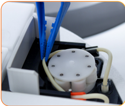
Figure 37 - Removing the pump tube
