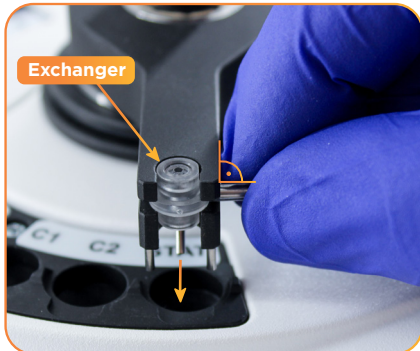
Figure 35- pull out exchanger
