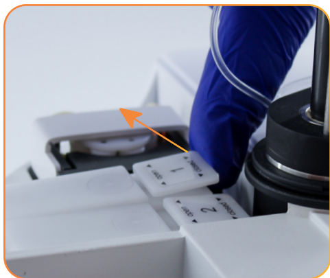
Figure 12 - Opening the sensor holder
